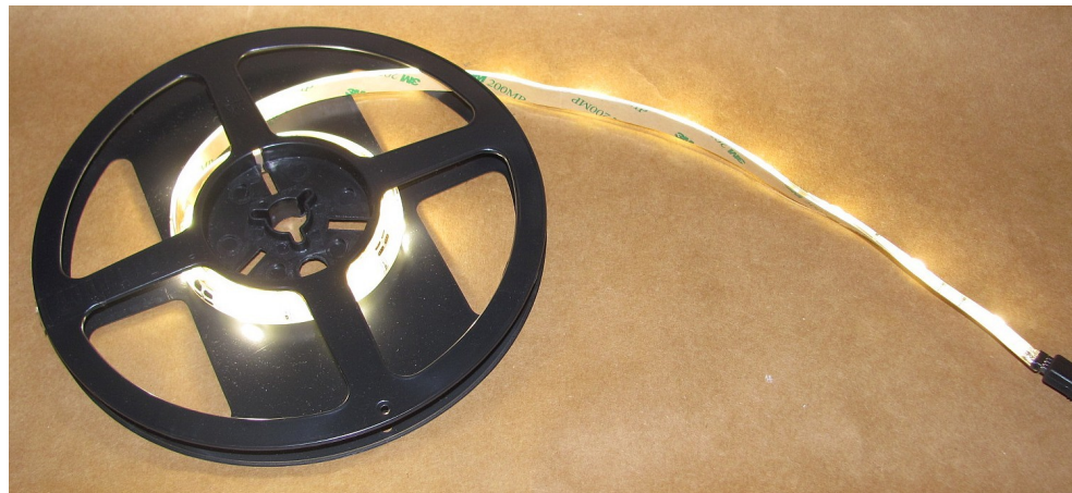
The LEDs come wound onto a reel to reel tape recorder style wheel. Here seen with one 1 metre length to demonstrate the flexibility of the strips (at least in one direction!).
